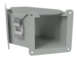
Hammond lay-in wireway fitting, 90-degree elbow, 4 x 4in, top opening, carbon steel, ANSI 61 gray, powder coat finish, quick-release clamps, NEMA 12. For use with 1485 series wireway.
