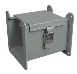
Hammond 1485 series lay-in wireway, 4 x 4 x 6in, carbon steel, ANSI 61 gray, powder coat finish, quick-release clamps, NEMA 12.
