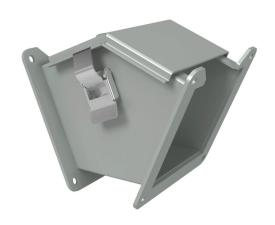
Hammond lay-in wireway fitting, 45-degree elbow, 4 x 4in, outside opening, carbon steel, ANSI 61 gray, powder coat finish, quick-release clamps, NEMA 12. For use with 1485 series wireway.
