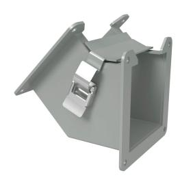
Hammond lay-in wireway fitting, 45-degree elbow, 4 x 4in, inside opening, carbon steel, ANSI 61 gray, quick-release clamps, NEMA 12.
