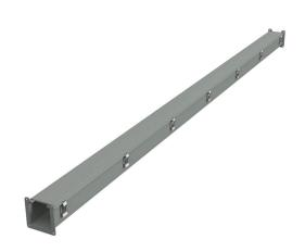
Hammond 1485 series lay-in wireway, 4 x 4 x 120in, carbon steel, ANSI 61 gray, powder coat finish, quick-release clamps, NEMA 12.
