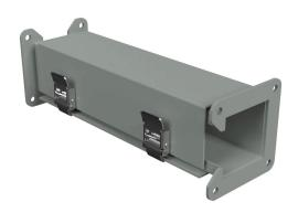
Hammond lay-in wireway fitting, clockwise transposition, 2.5 x 2.5in, carbon steel, ANSI 61 gray, quick-release clamps, NEMA 12.
