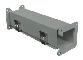
Hammond lay-in wireway fitting, clockwise transposition,  $2.5 \times 2.5$ in, carbon steel, ANSI 61 gray, powder coat finish, quick-release clamps, NEMA 12. For use with 1485 series wireway.
