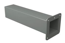
Hammond pull-through wireway fitting, cut-off fitting,  $2.5 \times 2.5 \times 12$  up to 12in, carbon steel, ANSI 61 gray, powder coat finish, NEMA 12. For use with 1485 series wireway.
