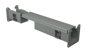
Hammond lay-in wireway fitting, cut-off fitting, 2.5 x 2.5 x 9 to 15in, carbon steel, ANSI 61 gray, powder coat finish, quick-release clamps, NEMA 12. For use with 1485 series wireway.
