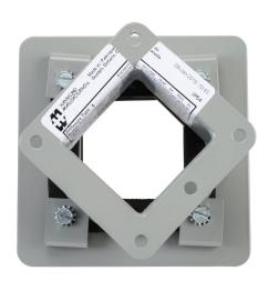
Hammond pull-through wireway fitting, box entry swivel nipple,  $2.5 \times 2.5 \times 2.25$ in, carbon steel, ANSI 61 gray, powder coat finish, NEMA 12. For use with 1485 series wireway.
