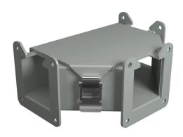
Hammond lay-in wireway fitting, tee, 2.5 x 2.5in, top opening, carbon steel, ANSI 61 gray, powder coat finish, quick-release clamps, NEMA 12. For use with 1485 series wireway.
