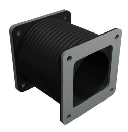
Hammond pull-through wireway fitting, flexible fitting, 2.5 x 2.5 x 3 to 10in, GortiflexTM bellows with carbon steel flanges, ANSI 61 gray, powder coat finish, NEMA 12. For use with 1485 and 1487 series wireway.
