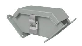
Hammond lay-in wireway fitting, 90-degree elbow, 2.5 x 2.5in, outside opening, carbon steel, ANSI 61 gray, powder coat finish, quick-release clamps, NEMA 12. For use with 1485 series wireway.
