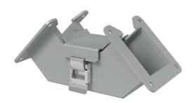
Hammond lay-in wireway fitting, 90-degree elbow, 2.5 x 2.5in, inside opening, carbon steel, ANSI 61 gray, powder coat finish, quick-release clamps, NEMA 12. For use with 1485 series wireway.
