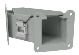
Hammond lay-in wireway fitting, 90-degree elbow, 2.5 x 2.5in, top opening, carbon steel, ANSI 61 gray, powder coat finish, quick-release clamps, NEMA 12. For use with 1485 series wireway.
