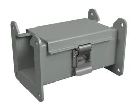
Hammond 1485 series lay-in wireway,  $2.5 \times 2.5 \times 6$ in, carbon steel, ANSI 61 gray, powder coat finish, quick-release clamps, NEMA 12.
