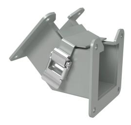
Hammond lay-in wireway fitting, 45-degree elbow, 2.5 x 2.5in, inside opening, carbon steel, ANSI 61 gray, powder coat finish, quick-release clamps, NEMA 12. For use with 1485 series wireway.
