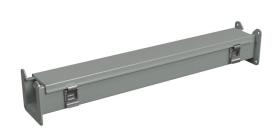
Hammond 1485 series lay-in wireway,  $2.5 \times 2.5 \times 24$ in, carbon steel, ANSI 61 gray, powder coat finish, quick-release clamps, NEMA 12.
