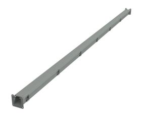
Hammond 1485 series lay-in wireway, 2.5 x 2.5 x 120in, carbon steel, ANSI 61 gray, powder coat finish, quick-release clamps, NEMA 12.
