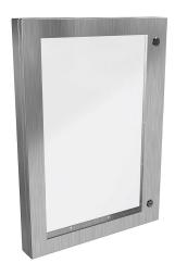
Hammond universal deep-hinged door, NEMA 4/4X/12, 28.19  $\times$  20.14  $\times$  2.75in, 316L stainless steel, concealed hinges, polycarbonate window. For use with wall-mount enclosures.
