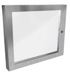
Hammond universal deep-hinged door, NEMA 4/4X/12, 22.19 x 26.14 x 2.75in, 316L stainless steel, concealed hinges, polycarbonate window. For use with wall-mount enclosures.
