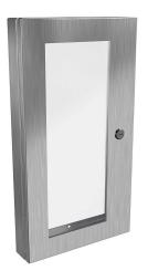
Hammond universal deep-hinged door, NEMA 4/4X/12, 22.19 x 12.14 x 2.75in, 316L stainless steel, concealed hinges, polycarbonate window. For use with wall-mount enclosures.
