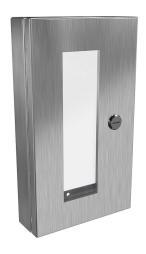
Hammond universal deep-hinged door, NEMA 4/4X/12, 14.19  $\times$  8.14  $\times$  2.75in, 316L stainless steel, concealed hinges, polycarbonate window. For use with wall-mount enclosures.
