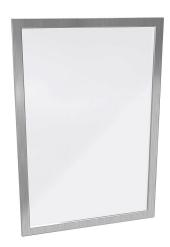
Hammond enclosure window, 29.00 x 19.00in window, UV-resistant polycarbonate, 31.63 x 21.63in frame, 304 stainless steel, #4 brush finish, oil-resistant neoprene gasket. For use with NEMA 4X enclosures. Mounting hardware included.
