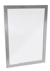
Hammond enclosure window, 23.00 x 15.00in window, UV-resistant polycarbonate, 25.63 x 17.63in frame, 304 stainless steel, #4 brush finish, oil-resistant neoprene gasket. For use with NEMA 4X enclosures. Mounting hardware included.
