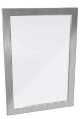
Hammond enclosure window, 17.00 x 11.00in window, UVresistant polycarbonate, 19.63 x 13.63in frame, 304 stainless steel, #4 brush finish, oil-resistant neoprene gasket. For use with NEMA 4X enclosures. Mounting hardware included.
