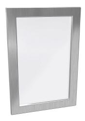
Hammond enclosure window, 13.00 x 8.00in window, UV-resistant polycarbonate, 15.63 x 10.63in frame, 304 stainless steel, #4 brush finish, oil-resistant neoprene gasket. For use with NEMA 4X enclosures. Mounting hardware included.
