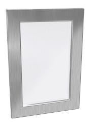
Hammond enclosure window, 9.00 x 5.50in window, UV-resistant polycarbonate, 11.63 x 8.13in frame, 304 stainless steel, #4 brush finish, oil-resistant neoprene gasket. For use with NEMA 4X enclosures. Mounting hardware included.
