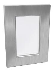
Hammond enclosure window, 5.00 x 3.00in window, UV-resistant polycarbonate, 7.63 x 5.63in frame, 304 stainless steel, #4 brush finish, oil-resistant neoprene gasket. For use with NEMA 4X enclosures. Mounting hardware included.
