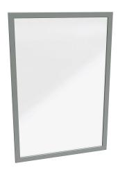
Hammond enclosure window, 35.00 x 23.00in window, UV-resistant polycarbonate, 37.63 x 25.63in frame, carbon steel, ANSI 61 gray, powder coat finish, oil-resistant neoprene gasket. For use with NEMA 4 enclosures. Mounting hardware included.
