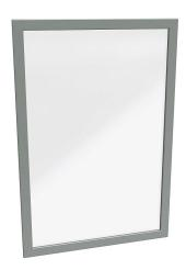
Hammond enclosure window, 29.00 x 19.00in window, UV-resistant polycarbonate, 31.63 x 21.63in frame, carbon steel, ANSI 61 gray, powder coat finish, oil-resistant neoprene gasket. For use with NEMA 4 enclosures. Mounting hardware included.
