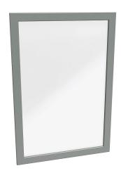
Hammond enclosure window, 23.00 x 15.00in window, UV-resistant polycarbonate, 25.63 x 17.63in frame, carbon steel, ANSI 61 gray, powder coat finish, oil-resistant neoprene gasket. For use with NEMA 4 enclosures. Mounting hardware included.
