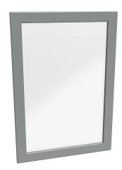
Hammond enclosure window, 17.00 x 11.00in window, UV-resistant polycarbonate, 19.63 x 13.63in frame, carbon steel, ANSI 61 gray, powder coat finish, oil-resistant neoprene gasket. For use with NEMA 4 enclosures. Mounting hardware included.
