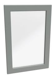
Hammond enclosure window, 13.00 x 8.00in window, UV-resistant polycarbonate, 15.63 x 10.63in frame, carbon steel, ANSI 61 gray, powder coat finish, oil-resistant neoprene gasket. For use with NEMA 4 enclosures. Mounting hardware included.
