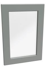
Hammond enclosure window, 9.00 x 5.50in window, UV-resistant polycarbonate, 11.63 x 8.13in frame, carbon steel, ANSI 61 gray, powder coat finish, oil-resistant neoprene gasket. For use with NEMA 4 enclosures. Mounting hardware included.
