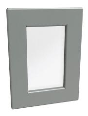
Hammond enclosure window, 5.00 x 3.00in window, UV-resistant polycarbonate, 7.63 x 5.63in frame, carbon steel, ANSI 61 gray, powder coat finish, oil-resistant neoprene gasket. For use with NEMA 4 enclosures. Mounting hardware included.
