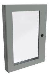
Hammond universal deep-hinged door, NEMA 4/12, 22.19 x 16.14 x 2.75in, carbon steel, ANSI 61 gray, concealed hinges, polycarbonate window. For use with wall-mount enclosures.
