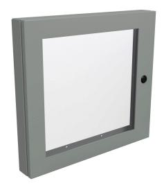
Hammond universal deep-hinged door, NEMA 4/12,  $18.19 \times 20.14 \times 2.75$ in, carbon steel, ANSI 61 gray, concealed hinges, polycarbonate window. For use with wall-mount enclosures.
