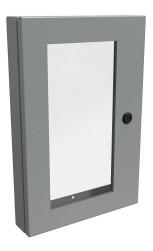
Hammond universal deep-hinged door, NEMA 4/12, 18.19 x 12.14 x 2.75in, carbon steel, ANSI 61 gray, concealed hinges, polycarbonate window. For use with wall-mount enclosures.
