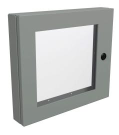
Hammond universal deep-hinged door, NEMA 4/12, 14.19  $\times$  16.14  $\times$  2.75in, carbon steel, ANSI 61 gray, concealed hinges, polycarbonate window. For use with wall-mount enclosures.
