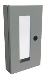
Hammond universal deep-hinged door, NEMA 4/12,  $14.19 \times 8.14 \times 2.75$ in, carbon steel, ANSI 61 gray, concealed hinges, polycarbonate window. For use with wall-mount enclosures.
