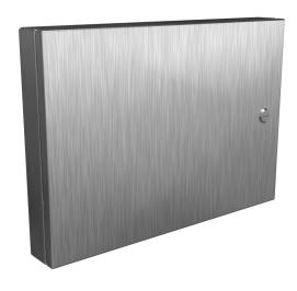
Hammond universal deep-hinged door, NEMA 4/4X/12, 14.19  $\times$  20.14  $\times$  2.75in, 316L stainless steel, concealed hinges. For use with wall-mount enclosures.
