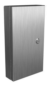
Hammond universal deep-hinged door, NEMA 4/4X/12, 14.19  $\times$  8.14  $\times$  2.75in, 316L stainless steel, concealed hinges. For use with wall-mount enclosures.
