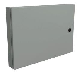
Hammond universal deep-hinged door, NEMA 4/12, 14.19  $\times$  20.14  $\times$  2.75in, carbon steel, ANSI 61 gray, concealed hinges. For use with wall-mount enclosures.
