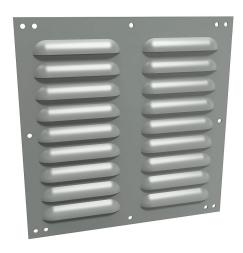
Hammond louver vent, 10.56 x 10.50in (HxW), carbon steel, ANSI 61 gray, powder coat finish, for ventilation of metal enclosure. Mounting hardware included.
