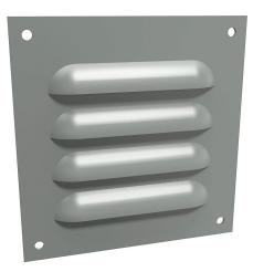
Hammond louver vent, 5.62 x 5.50in (HxW), carbon steel, ANSI 61 gray, powder coat finish, for ventilation of metal enclosure. Mounting hardware included.
