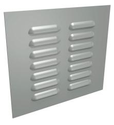
Hammond louver vent assembly, 9.00 x 10.30in (HxW), carbon steel, ANSI 61 gray, powder coat finish, 6.25 x 7.75in (HxW) cutout, for ventilation of metal enclosure. Aluminum filter mesh and mounting hardware included.
