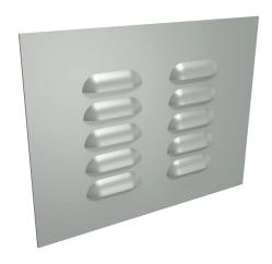
Hammond louver vent assembly,  $6.40 \times 8.30$ in (HxW), carbon steel, ANSI 61 gray, powder coat finish,  $3.50 \times 5.75$ in (HxW) cutout, for ventilation of metal enclosure. Aluminum filter mesh and mounting hardware included.
