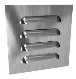
Hammond louver vent assembly,  $6.40 \times 6.30$ in (HxW), 304 stainless steel,  $4.00 \times 3.75$ in (HxW) cutout, for ventilation of metal enclosure. Aluminum filter mesh and mounting hardware included.
