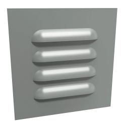
Hammond louver vent assembly, 6.40 x 6.30in (HxW), carbon steel, ANSI 61 gray, powder coat finish, 4.00 x 3.75in (HxW) cutout, for ventilation of metal enclosure. Aluminum filter mesh and mounting hardware included.
