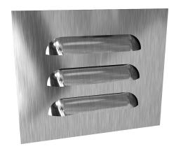
Hammond louver vent assembly,  $5.30 \times 6.30$  in (HxW), 304 stainless steel,  $2.88 \times 3.75$  in (HxW) cutout, for ventilation of metal enclosure. Aluminum filter mesh and mounting hardware included.
